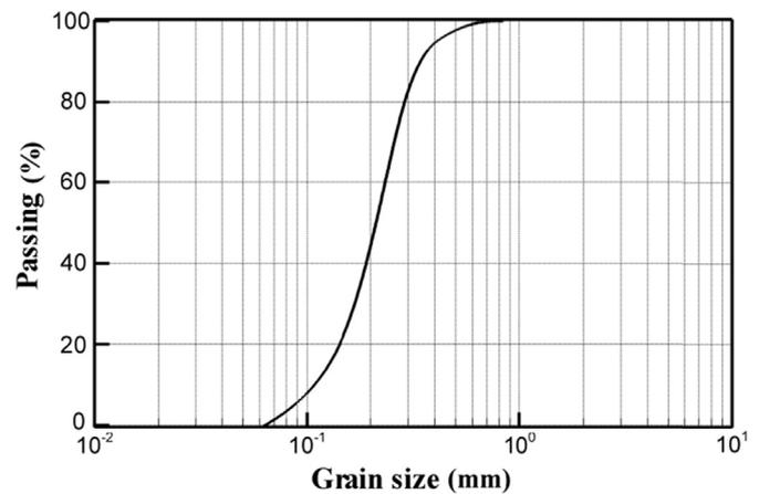
Fig. 1. Particle size distribution curve for Babolsar sand.
