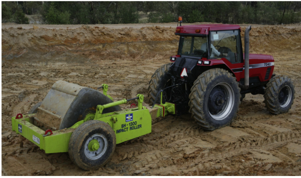
Fig. 1. The 4-sided impact roller and tractor.
