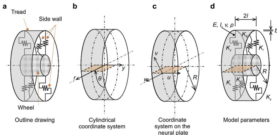
Fig. 1. A three-dimensional flexible ring-based model for the tire.
