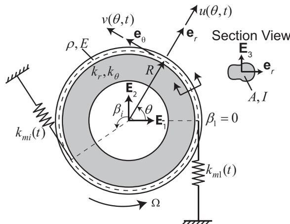
**Fig. 1.** Schematic of the rotating, elastic ring model with an arbitrary number of space-fixed, fluctuating discrete stiffnesses. The  $\{\mathbf{E}_1, \mathbf{E}_2\}$  basis is fixed in space. The radial ( $u$ ) and tangential ( $v$ ) deformations are measured with respect to the stationary, cylindrical  $\{\mathbf{e}_r, \mathbf{e}_\theta\}$  basis.
