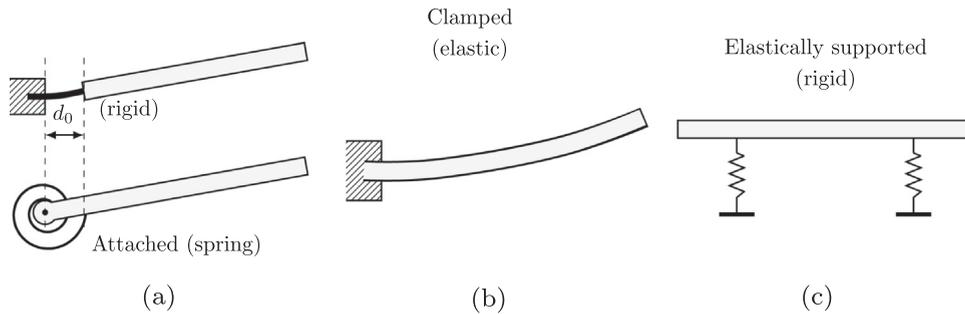
**Fig. 1.** Sketch of the mechanical system consisting of a rigid planar beam attached to one end of a flat spring (a), a thin elastic one-dimensional planar beam clamped to one end (b), a suspended rigid planar beam (c).
