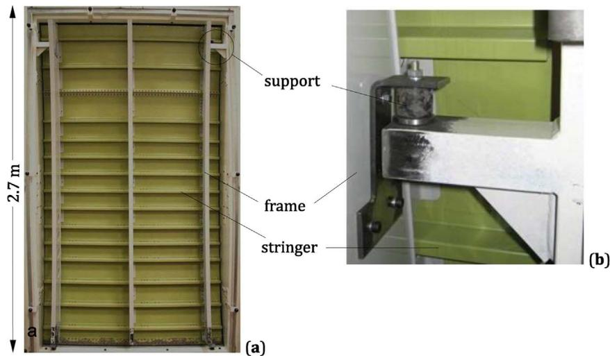
Fig. 1. Aircraft panel test bed, adapted from [9].
