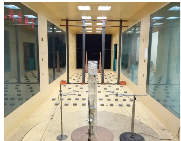
Fig. 1. Rigid model pressure measurement wind tunnel test.
