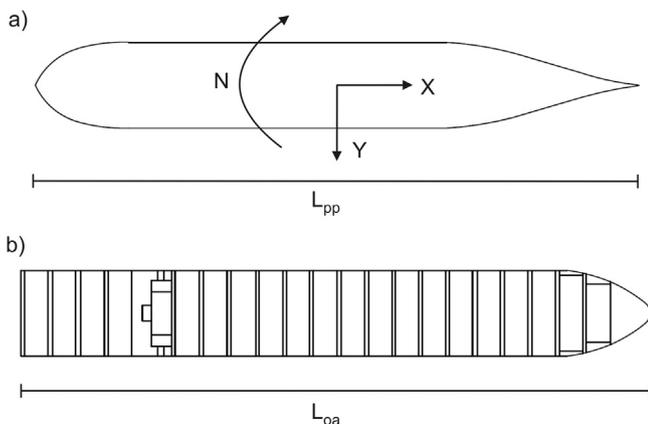
**Fig. 1.** a) Definition of forces X and Y, and moment N. The origin is located halfway the length between perpendiculars ( $L_{pp}$ ) here based on the hull at the waterline b) Top view of the ship, showing the length over all ( $L_{oa}$ ).
