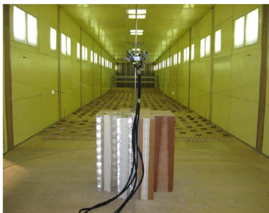
(a) Crucifix-form building model in boundary layer wind tunnel
