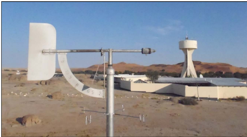
Fig. 1. Pressure plate wind indicator at Gobabeb. Photo courtesy Mr Titus Shuuya (GRTC).
