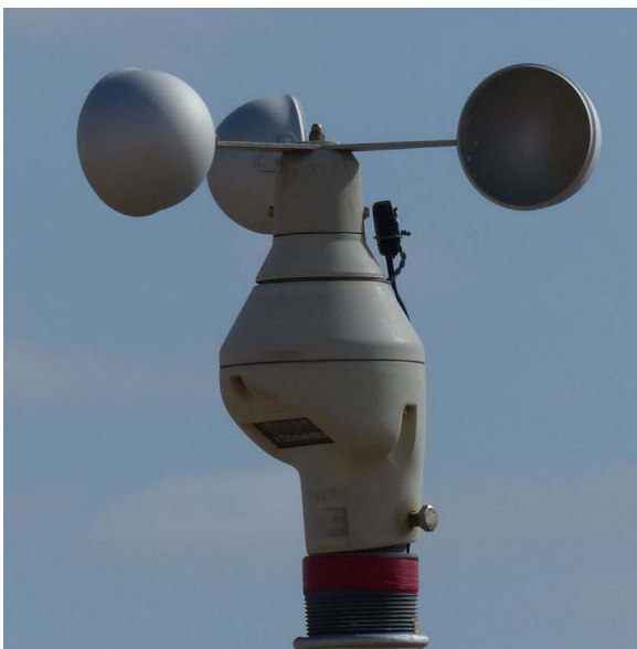
Fig. 2. Mechanical wind totalizer at Gobabeb. Photo courtesy Dr Roland Vogt (University of Basel).
