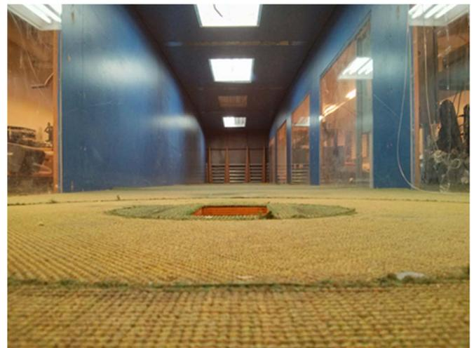
Fig. 3. View of Test Section and Upstream Fetch of Atmospheric Boundary Layer Wind Tunnel at Concordia University.
