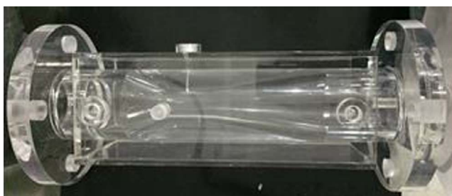
Fig. 2. Configuration of the venturi-type bubble generator with the additional square glass box.
