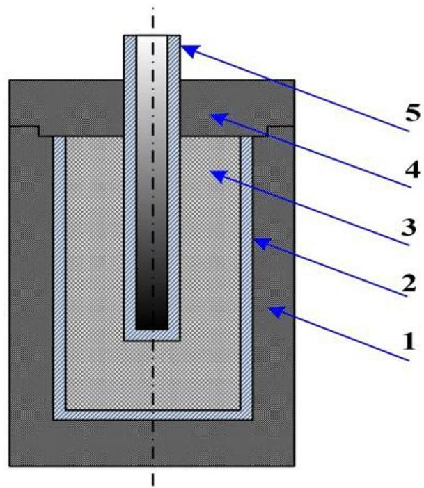
Fig. 1. Scheme of preparing the assembly of the melting unit for annealing: 1 – graphite crucible; 2 – tantalum glass; 3 – foam graphite; 4 – crucible cover; 5 – tantalum casing of thermometry system.
