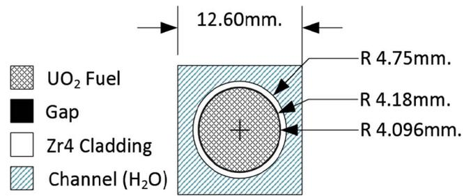
Fig. 1. Single pellet channel initial geometry.
