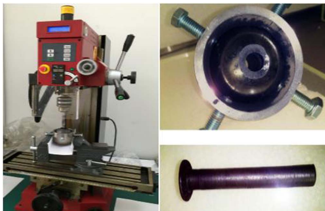
Fig. 1. Drilling machine with a special annular drill and cylindrical graphite stick sample of the irradiated graphite sphere of HTR-10.
