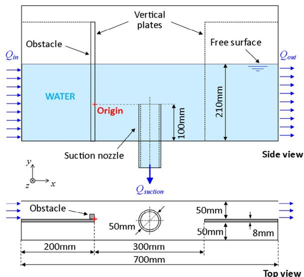
Fig. 1. Test section of the rig BANGA. The top picture is the side view and the bottom one is the top view. The origin of the Cartesian frame is indicated with a cross.  $Q_{in}$  and  $Q_{out}$  denote the inlet and outlet flow rates, respectively.
