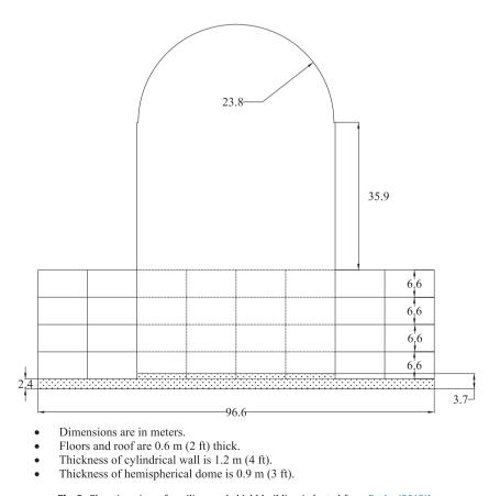
Fig. 2. Elevation view of auxiliary and shield building (adapted from Roche (2013)).
