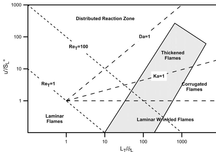
Fig. 1. Borghi diagram with four combustion regimes. The relevant region of nuclear power plant accidents according to Faix-Gantier (2001) is colored in gray.
