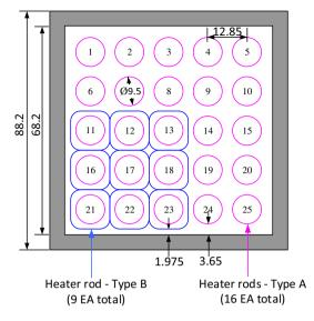
Fig. 2. Cross-sectional view of the partially-blocked rod bundle (unit: mm).
