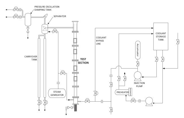
Fig. 1. Schematic diagram of the reflood test facility.
