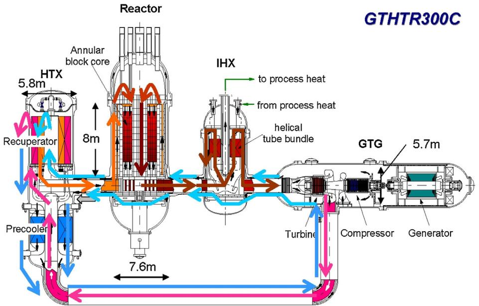
Fig. 1. Schematic of GTHTR300C.
