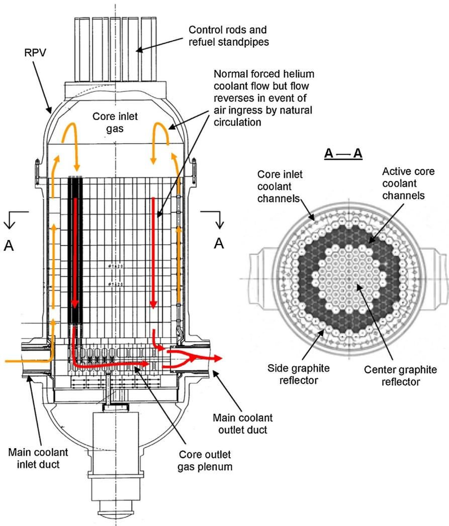
Fig. 2. Flow path in GTHTR300C.
