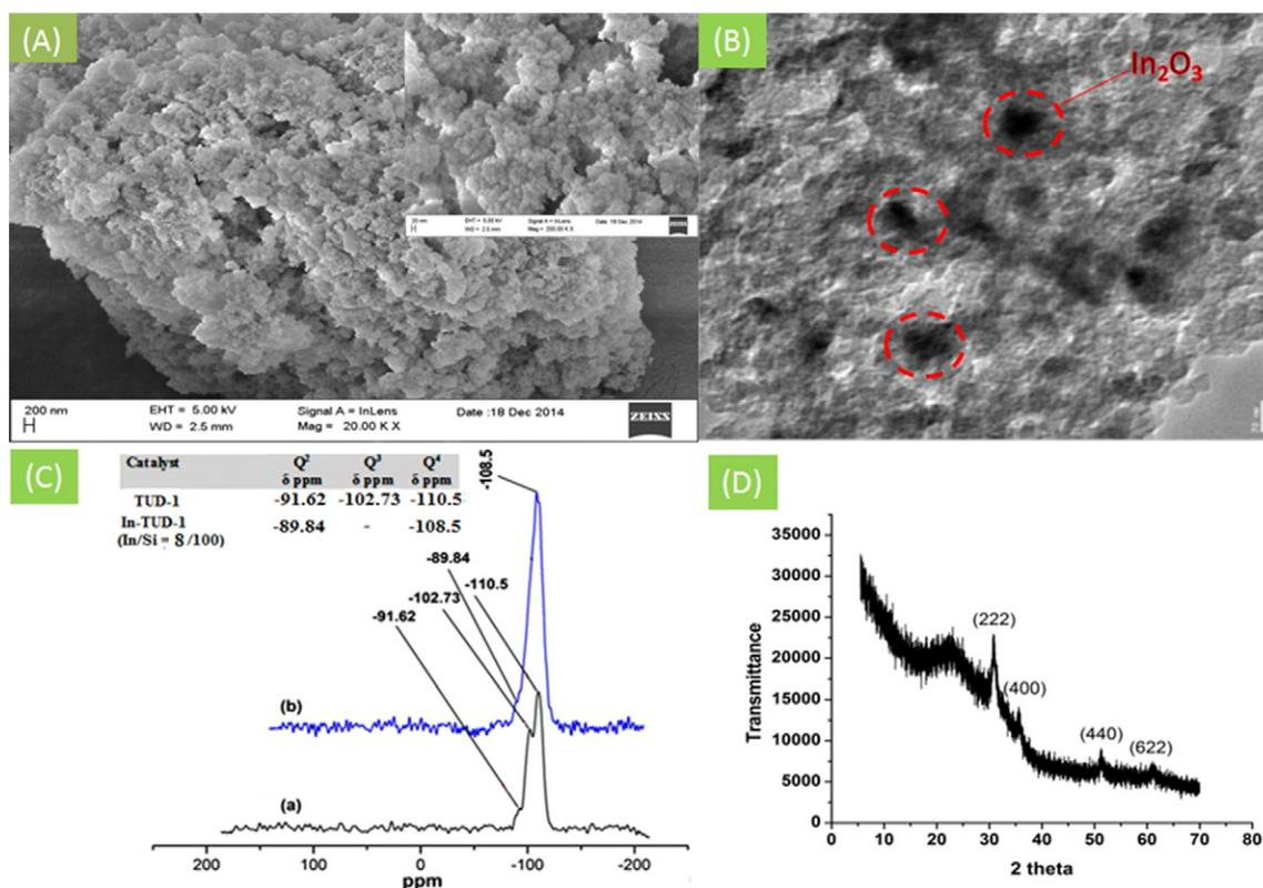
Fig. 1. (A) FESEM image of InO<sub>x</sub>/TUD-1 (In/Si = 8/100) viewed at 200 nm and 20 nm (inset) (B) HRTEM image of InO<sub>x</sub>/TUD-1 (In/Si = 8/100) (C) <sup>29</sup>Si NMR of (a) TUD-1, (b) InO<sub>x</sub>/TUD-1 (In/Si = 8/100) and (D) XRD of InO<sub>x</sub>/TUD-1 (In/Si = 8/100).
