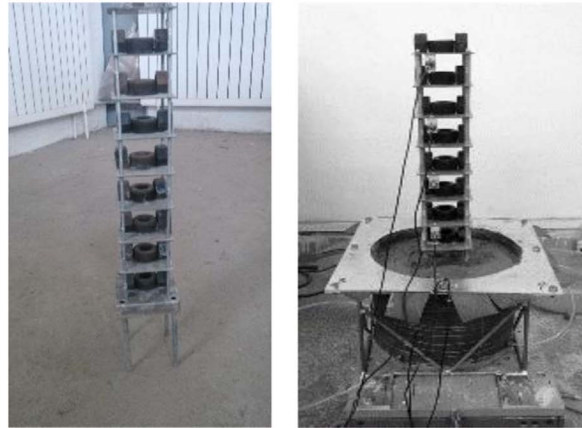
Fig. 1. Test model and loading system.
