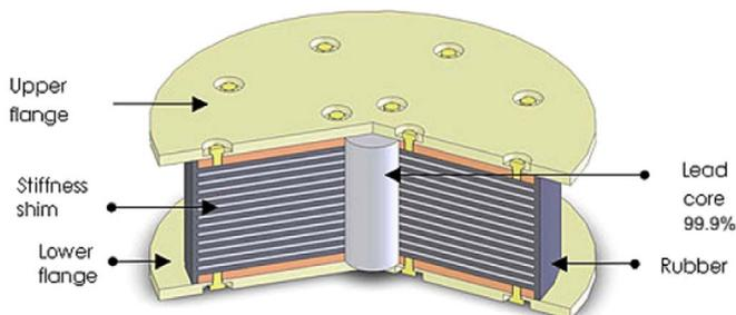
Fig. 2-1. Lead rubber bearing (LRB).
