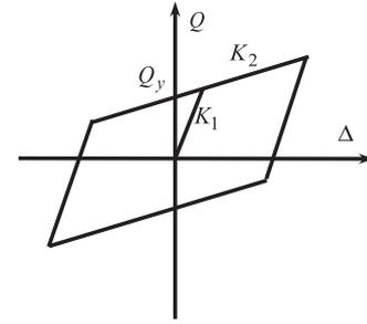
Fig. 2-2. LRB Load-deformation model.
