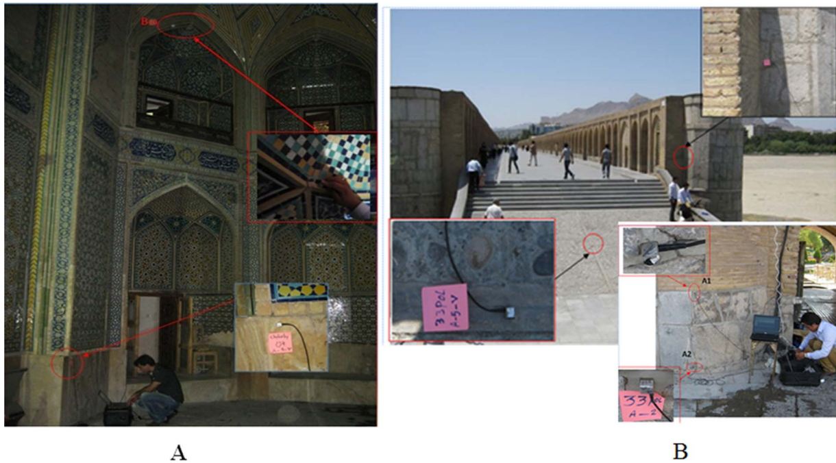
Fig. 2. Instrumented monumental buildings to measure vibration received by historical structures using FTA method, A) MCH, B) SSP.
