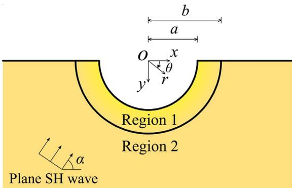
Fig. 1. Cross-section of a semi-cylindrical canyon with a radially inhomogeneous surface layer.
