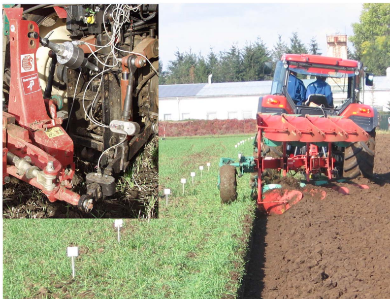
Fig. 1. Measurement of conventional right-handed ploughing with mechanically controlled, four furrow reversible mounted plough and the three-point hitch with strain gauge sensors.
