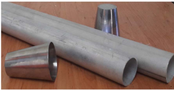
Fig. 1. Materials, capped-end steel cones and cylindrical aluminum tubes.
