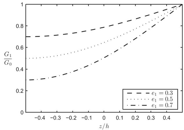
Fig. 1. Variation of shear modulus through the dimensionless thickness for nonlinear nonsymmetric pore distribution for different values of  $e_1$ .
