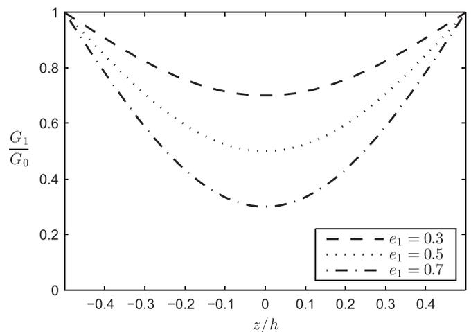
Fig. 2. Variation of shear modulus through the dimensionless thickness for nonlinear symmetric pore distribution for different values of  $e_1$ .
