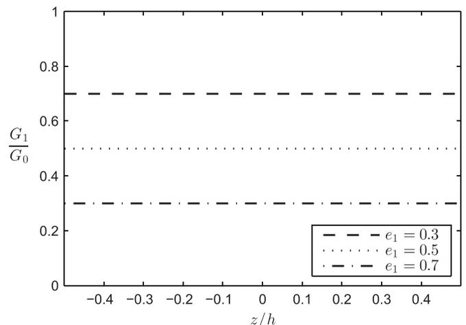
Fig. 3. Variation of shear modulus through the dimensionless thickness for monotonous pore distribution for different values of  $e_1$ .
