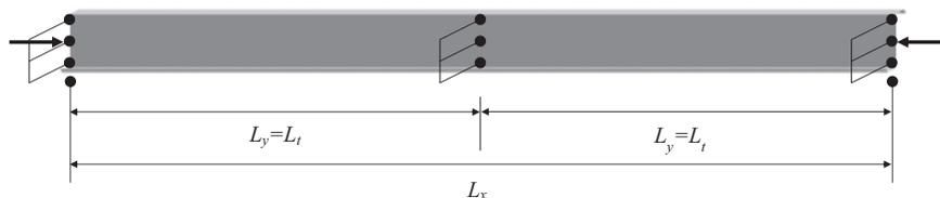
Fig. 1. Typical bracing configuration where unbraced lengths are different.
