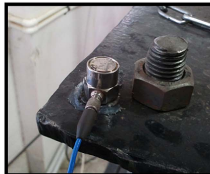
Fig. 4. Drop Hammer accelerometer sensors [26].
