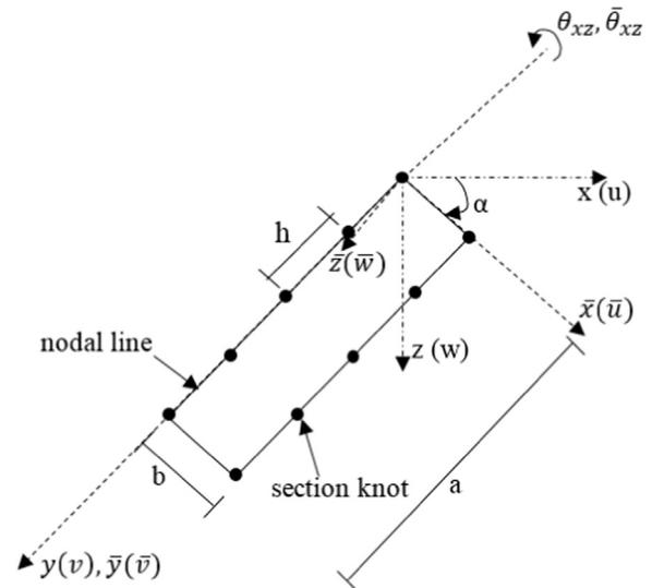
Fig. 1. Spline finite strip with coordinate axes.
