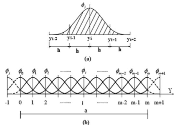
Fig. 2. (a) Local B3 spline (b) B3 spline series.
