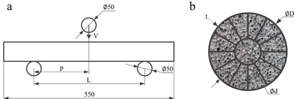
Fig. 1. Loading condition and cross section of FBTS: (a) Loading condition and (b) cross section.
