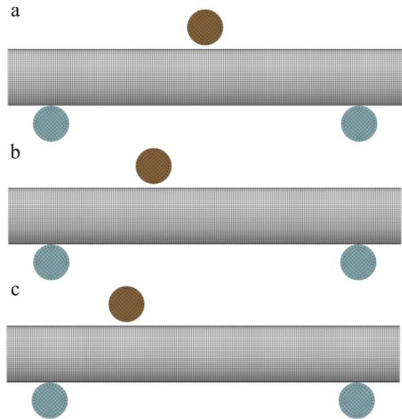
Fig. 2. Finite element models of FBTS with different punch positions: (a)  $p = L/2$ , (b)  $p = L/3$  and (c)  $p = L/4$ .
