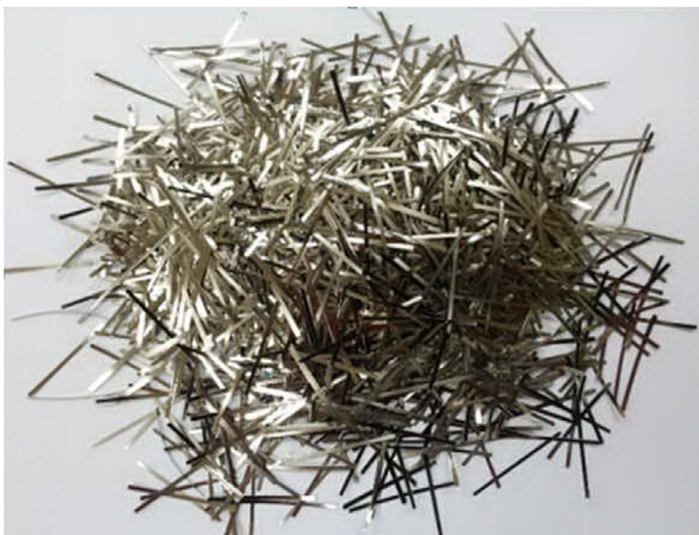
Fig. 1. Amorphous metallic fibers.
