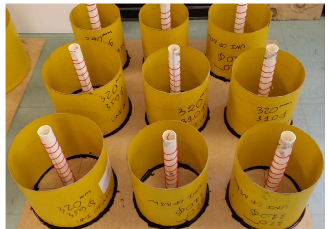
Fig. 2. Cardboard moulds with the internal diameters ranging from 150 mm to 508 mm.
