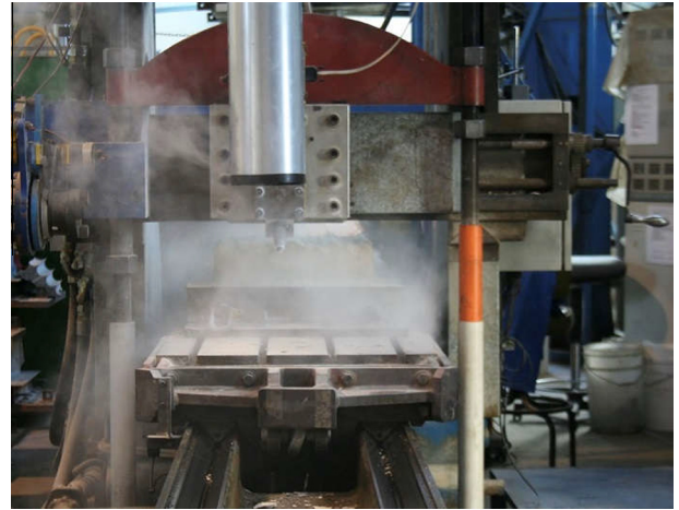
Fig. 2. Photograph of the linear rock cutting planer.
