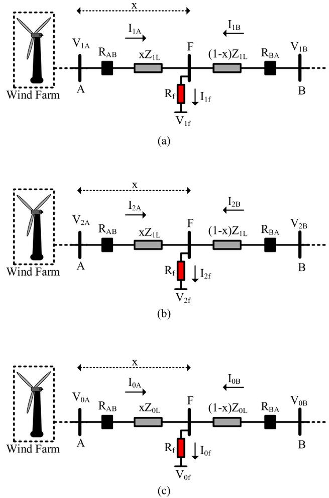
Fig. 2. Positive (a), negative (b) and zero-sequence (c) networks of the power system from the viewpoint of the  $R_{AB}$  relay for an A-G fault.
