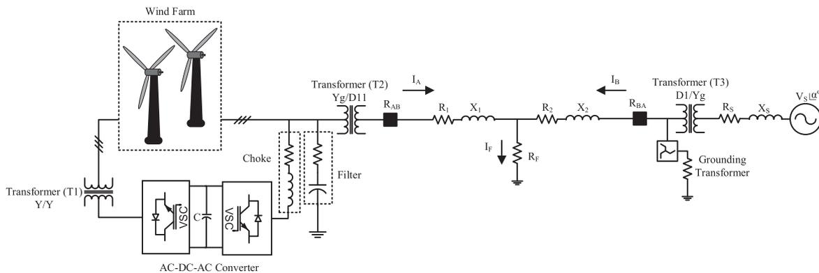
Fig. 1. Single-line diagram of power system with the wind farms.
