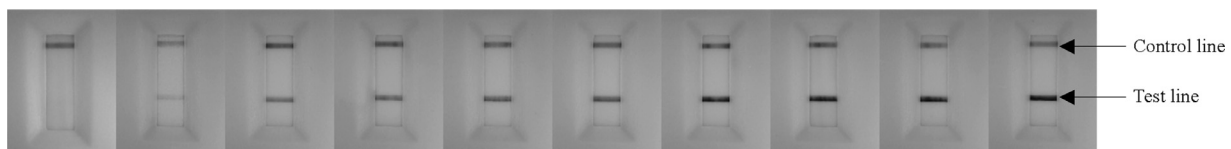
Fig. 2. Images of gold immunochromatographic strip with different concentration (from the left side: 0, 10, 35, 75, 100, 150, 200, 300, 400, 500 mIU/ml).
