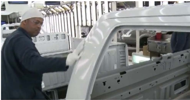
Fig. 1. Check-men working on a production line, inspecting car body parts following the painting stage (image courtesy of FORD Dearborn, USA).
