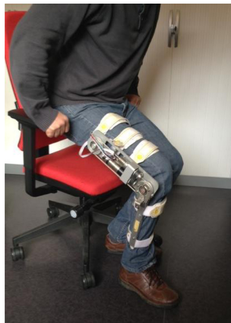
Fig. 1. EICoSi (Exoskeleton Intelligently Communicating and Sensitive to Intention) of LISSI laboratory worn by a healthy subject.
