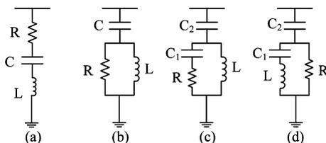
Fig. 1. Typical PPFs: (a) single-tuned filter, (b) second-order damped filter, (c) third-order damped filter, and (d) C-type damped filter.
