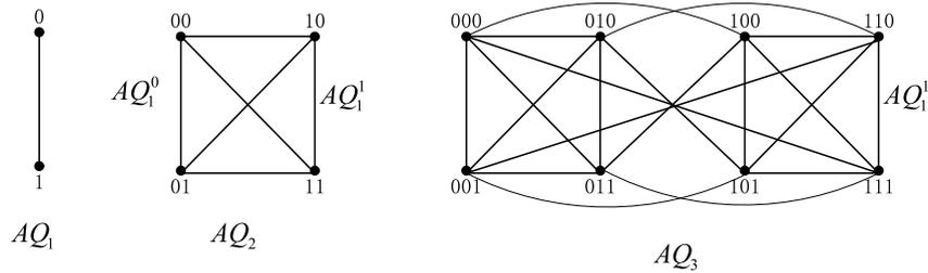
Fig. 1. Augmented cubes of dimensions 1, 2 and 3.
