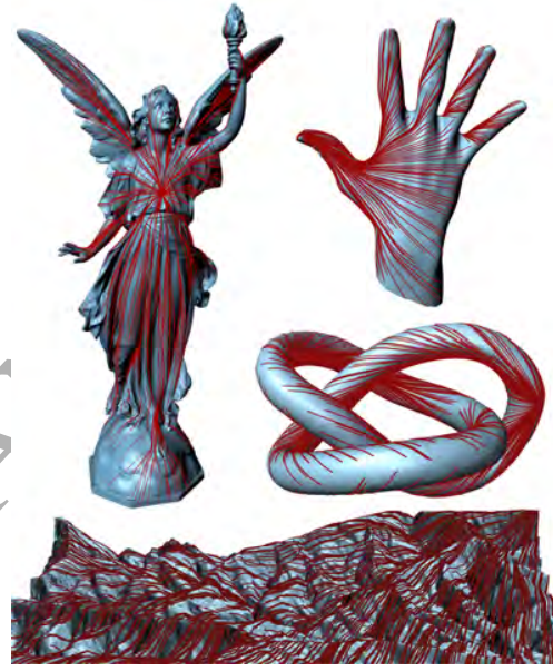
Figure 1: Geodesic paths computed using our FPP (Fast Path Propagation) algorithm. Herein, the Lucy model contains 14M vertices. Refer to the supplementary material for more results.
