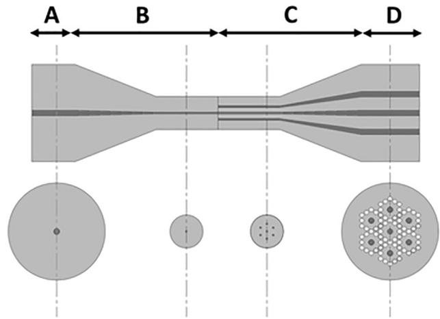
Fig. 2. Scheme of the tapered region and the splice between the SMF-28 and MCF-7 and cross-sections of the fiber's structure at points along the fiber taper. A- the SMF-28. B- the tapered SMF-28. C- the tapered MCF-7. D- the MCF-7. Dimensions on the scheme do not reflect real sizes.
