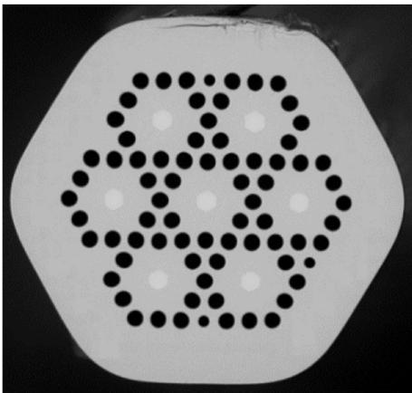
Fig. 1. Scanning electron microscope (SEM) image of MCF-7. The measured fiber dimensions are:  $d_{\text{core}} = 6.2 \mu\text{m}$ ,  $\Lambda = 7.6 \mu\text{m}$ ,  $d_{\text{hole}} = 5.6 \mu\text{m}$  and the clad diameters equal  $121 \mu\text{m}$  and  $130 \mu\text{m}$ .  $\text{GeO}_2$  doping of the core is 4% mol.
