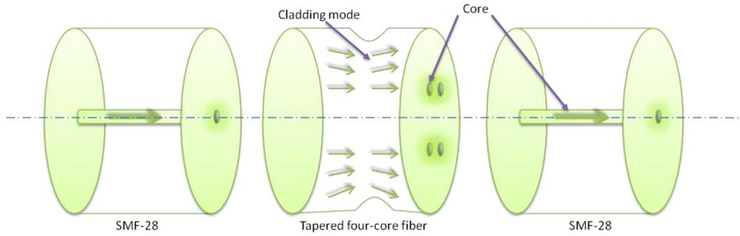
Fig. 1. Schematic diagram of SMF-TMCF-SMF structure with four core fiber.
