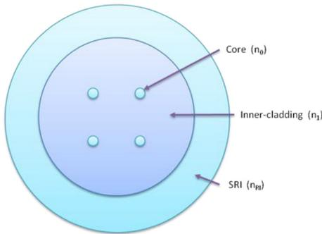
Fig. 2. Configuration of MCF model structure with double-cladding.
