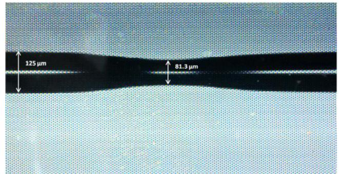
Fig. 4. The picture of tapered MCF.
