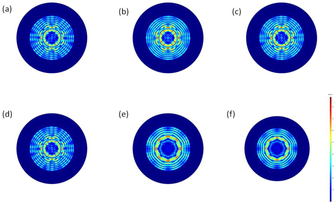
Fig. 3. Mode field distribution for inner cladding are obtained by using FEM with different SRI: (a) 1.33, (b) 1.34, (c) 1.35, (d) 1.36, (e) 1.37, (f) 1.38.
