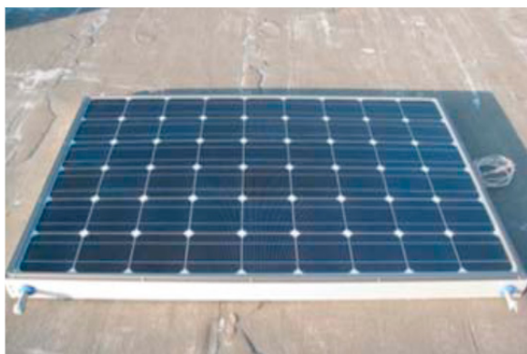
Fig. 1. Unglazed Polygeneration PVT collector
