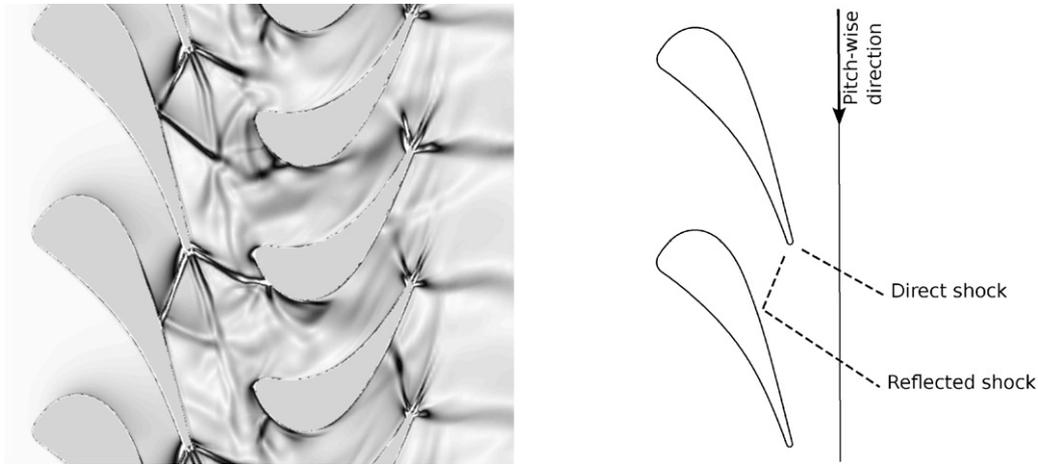
Fig. 1. (Left) Vane/rotor shock interaction (Paniagua et al. [7]). (Right) Plane of interest to assess vane downstream distortion.
