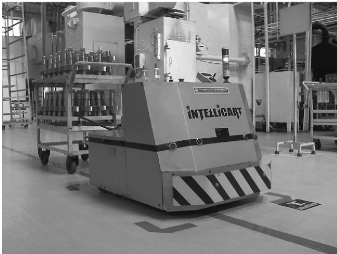
Fig. 1. An industrial path-following mobile robot.
