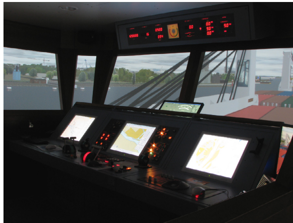
Fig. 1. Example of a bridge ship handling simulator ANS 6000 manufactured by RDE GmbH.
