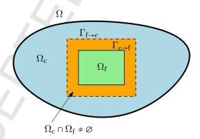
The proposed coupling method employs overlapping domain decomposition. This figure illustrates the partitioning of the computational domain  $\Omega$  into subdomains in which continuum-scale and pore-scale features are sought after.
