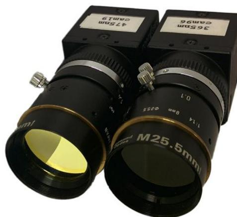
Fig. 3. Two-camera MSI system with custom optical filters.
