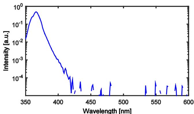
Fig. 1. Emission spectra of the 365 nm UV LED excitation light source.
